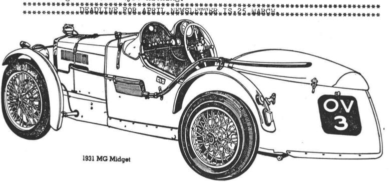
The English MG, one of America's favorite sports cars today and one of the most successful in road racing competition, was first built in 1923. The 1931 MG Midget, a small, open two-seater with pointed tail, was the Type C racing model. It had a four-cylinder, 37 h.p. engine, and sold for \$2700. In super-charged form, it was clocked at 103 mph on the Montlhery track near Paris and that model became known as the 'Montlhery Midget.'"\*
