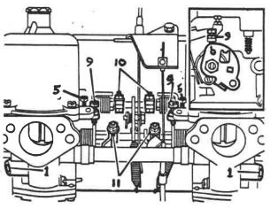
Before you start, warm up the engine to normal operating temperature, remove the air cleaner(s), slacken one of the clamping bolts on the throttle linkage (10) so that each carb throttle will work independently, and one of the clamping bolts on the choke linkage (11) so that each choke will work independently. That's step 1.
