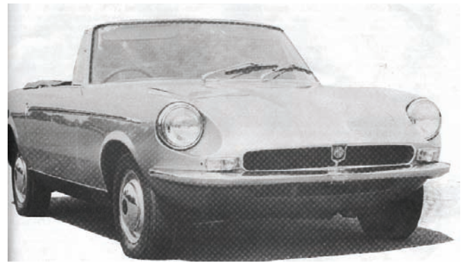
Grille, badge. Headlamp treatment, wipers, and marker lights appear to be off the shelf MGB pieces. Windshield looks like a B clone, and EX234's stance and lines give it an Italian flavor not too far removed from the Alfa/Fiat Spyder.
