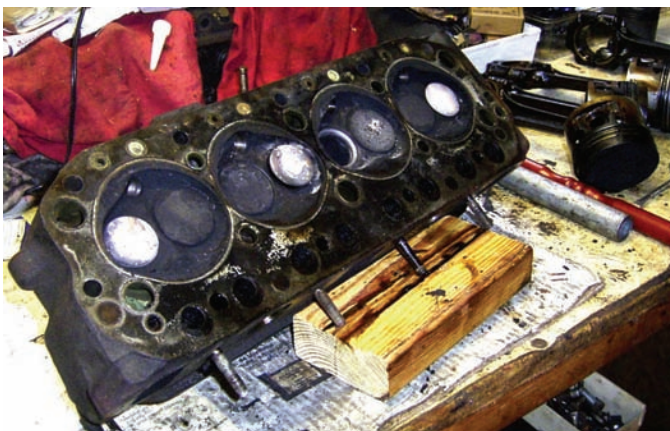
Carbon build up
