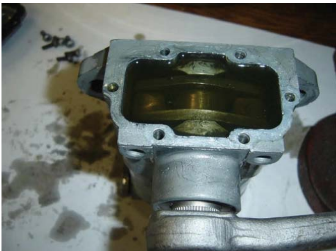
Flush reservoir, fill with oil of choice and replace lid. Top off through the filler bolt before installing
