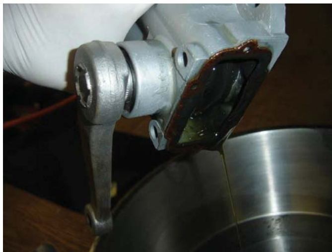
Drain the goop from the reservoir and wipe off as much surface as possible
