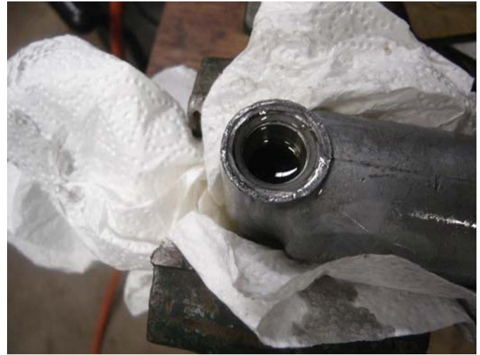
Fill, bleed, and reinstall valve. Center the lever arm to allow oil to fill valve chamber
