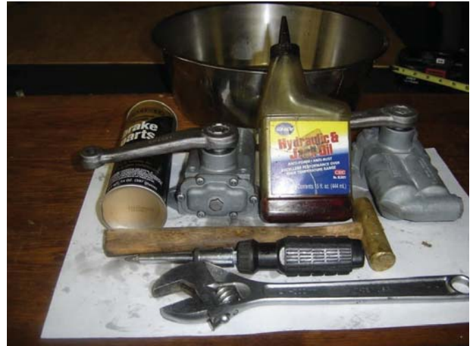
It doesn't take much in the way of materials to service shocks. A quart of 30wt non detergent oil is also required.
