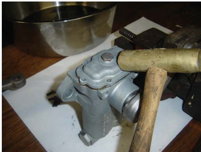
Gently tap lid off, careful not to tear cork gasket
