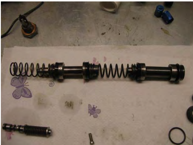
Primary and secondary pistons, Primary Diff. Piston ready for installation. Note the stop pin bottom center for retaining primary piston
