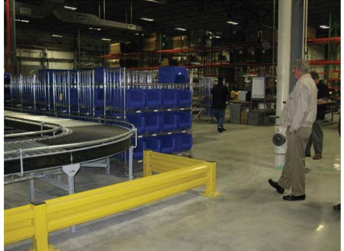
New conveyors and shipping equipment were installed for handling the products, with ergonomic considerations. In order to be efficient, parts with a higher frequency of orders are placed closer to the conveyors, as a means to save steps and time. Movement-sensitive lighting is currently in place in “critical” areas like the bathrooms to save electricity, and more are planned to be installed for use on the lower, darker shelving areas in order to improve visibility.
