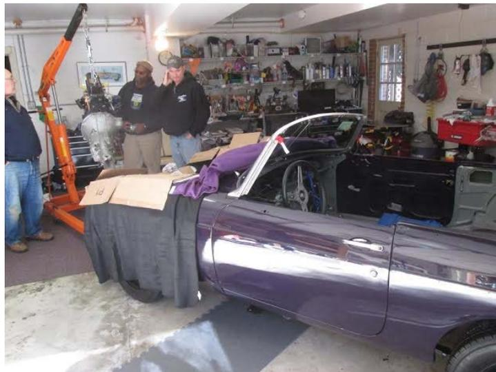
3. A “Leveler” is good money spent. It allows you to change the angle of the engine in degrees as you lower the “lump” into place. Just make sure you grease the thing so it doesn’t bind up.
