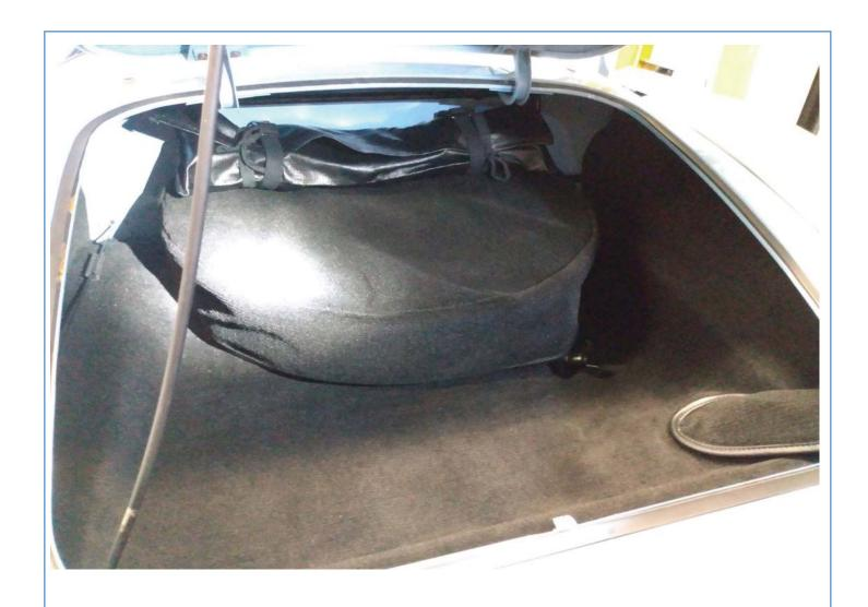
I just finished installing trunk carpet and a new tire cover in my MGA. I also re-painted the spare tire hold down clamp and added stock/original style straps and Jack storage bag. Probably took about 4 hours.
