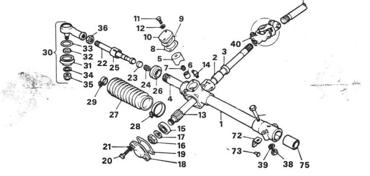
Removal of the steering shaft. item 13 in the diagram was not too difficult. Once the cap (18) was removed. the shaft, complete with bearing (15), could be knocked forward out of the rack housing. I had to cut away part of the front valance to get it all the way out. This, then, brings me to the point of this article. To my surprise, the gear and bearing were completely dry and a little rusty, as though the steering assembly had never been lubricated since the car left the factory 15 years ago!
