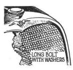
Two cooling system tips: (above) a true honeycomb radiator can be sealed by passing a long bolt, fitted with steel and rubber washers, through the leaking tube. (Right) Perished rubber connections may impede the flow of water and lead to overheating: badly fitting hose clips will often give rise to serious leaks,
