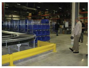
New conveyors and shipping equipment were installed for handling the products, with ergonomic considerations. In order to be efficient, parts with a higher frequency of orders are placed closer to the conveyors, as a means to save steps and time. Movement-sensitive lighting is currently in place in "critical" areas like the bathrooms to save electricity, and more are planned to be installed for use on the lower, darker shelving areas in order to improve visibility.
