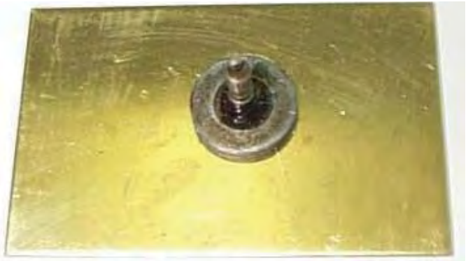
Fig. 4. Gear pressed into RTV
