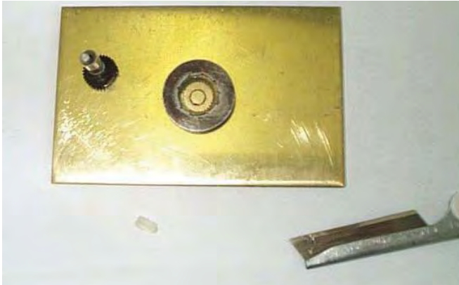
Fig. 7. Ready for epoxy and new teeth
