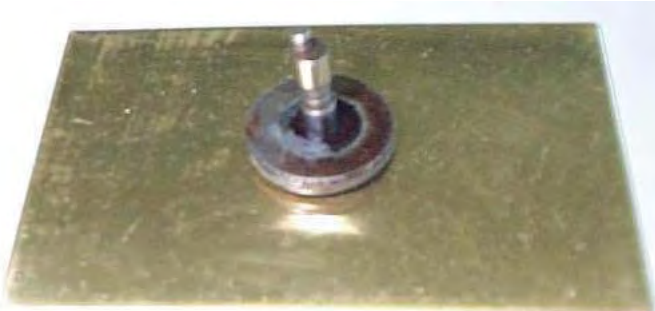
Fig. 8. Epoxy in place, molding new teeth
