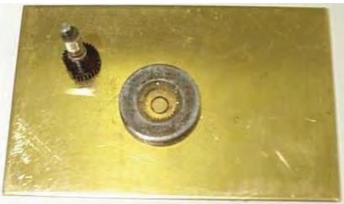
Fig. 5. Gear removed, mold formed
