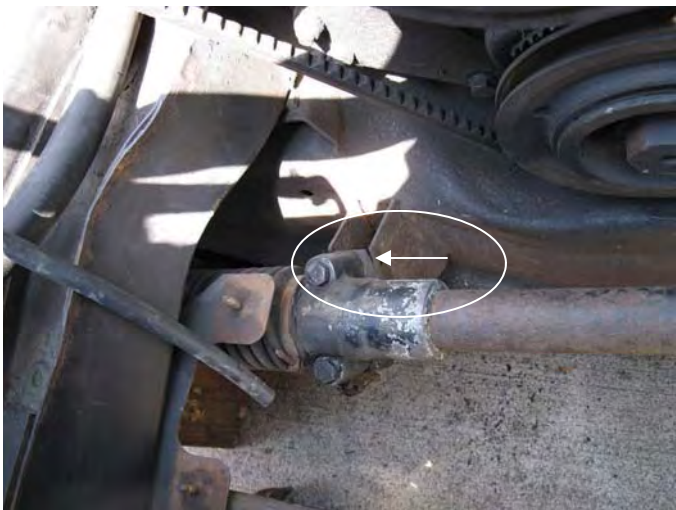
Bill's steering problem. Arrow shows crack on right side which was later welded during the session.
