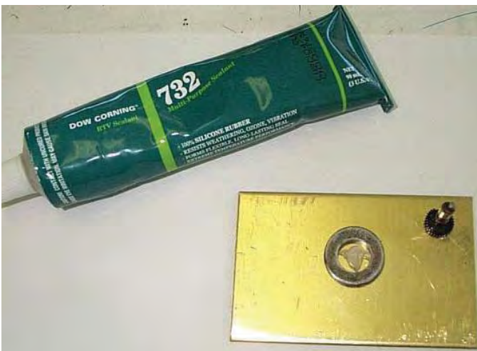
Fig. 3. RTV in place
