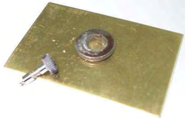
Fig. 9. Gear removed with new teeth
