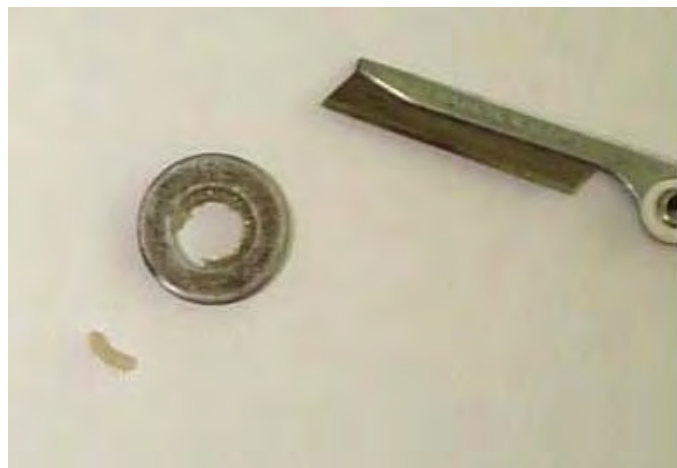
Fig. 6. Flat spot with no teeth cut away
