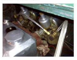
Folks, this was a lesson about not only some old fuel lines, but likely, the effects of ethanol on old rubber. Check your fuel lines and take action. The Moss Teflon-lined S.S. hoses are excellent. A potential catastrophe [engine fire] was narrowly averted.
