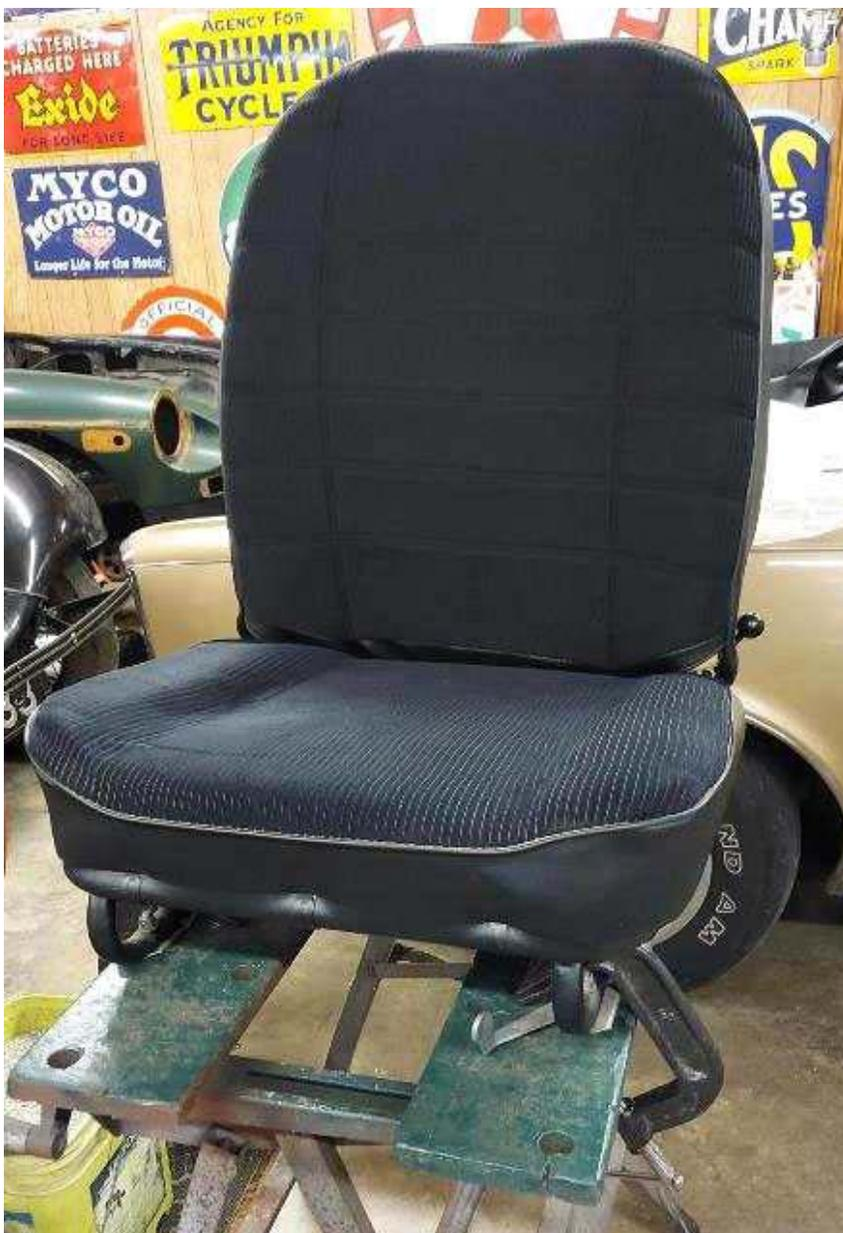
**Completed re-covering of seat back. Headrest has not been reinstalled yet.**
