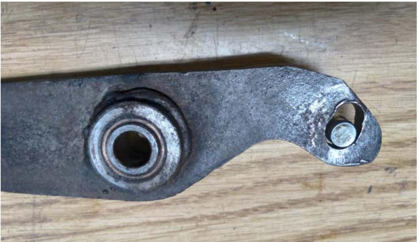
**Figure 1 - clutch pedal worn clevis pin hole**
