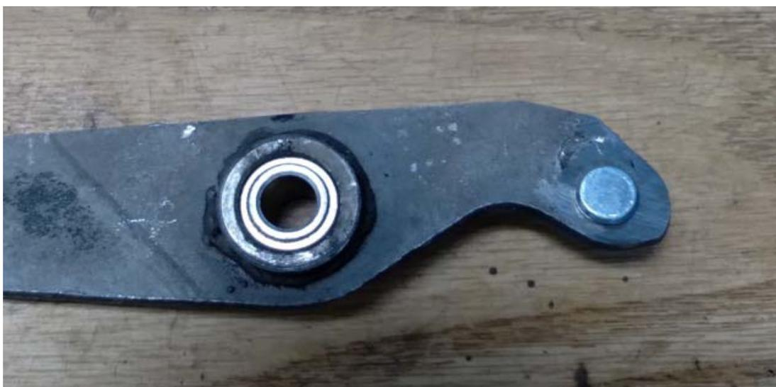
**Figure 2 - clutch pedal reworked**
