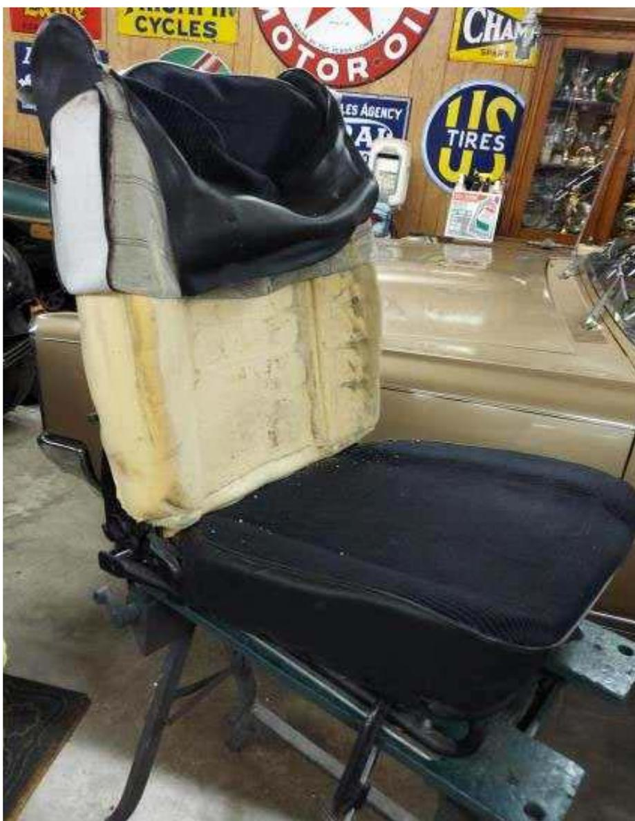
***MGB GT Seat mounted on portable workbench, held in place using C clamps. This photo shows old upholstery being removed carefully by rolling it up over the foam backing. Note headrest is removed.***
