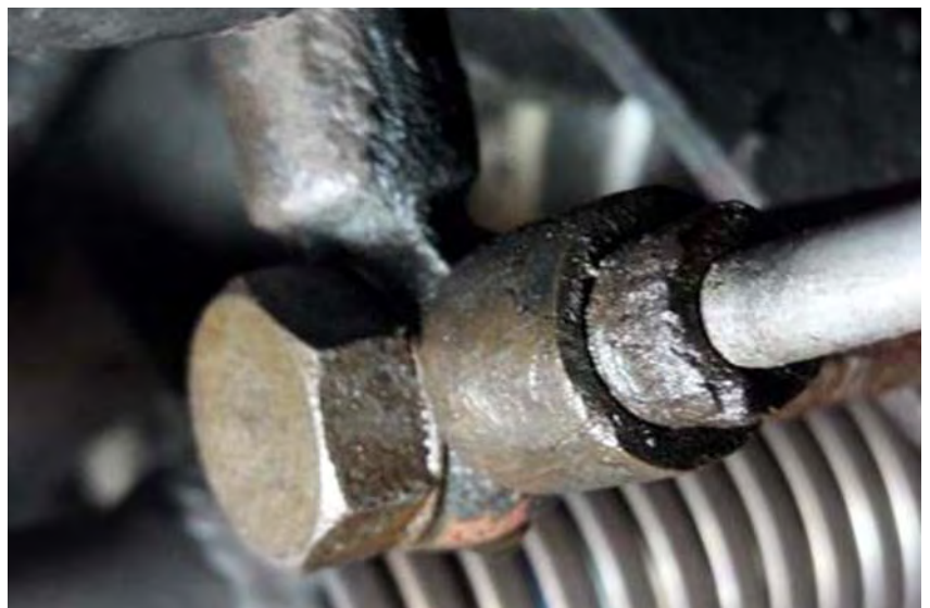
How not to tighten (or remove) a brake line nipple!
