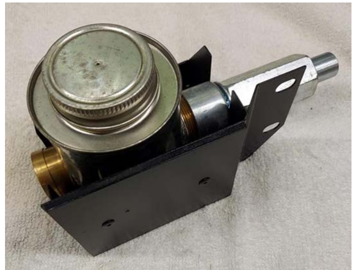
Our new Master Cylinder mounted in its protective “box” with heat shield. Note the two holes on the right side “mounting flange.” But, what does it mount to? The bracket attached to the car frame where the Master Cylinder attaches showed no holes corresponding to those on the flange on this “box” until I scraped away some old paint.
