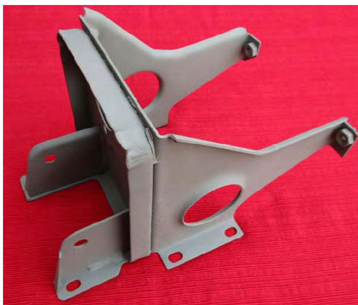
Framework supporting both brake and clutch master cylinders.
