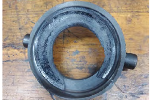
Badly worn throwout bearing. Note the missing chunk at the bottom.
