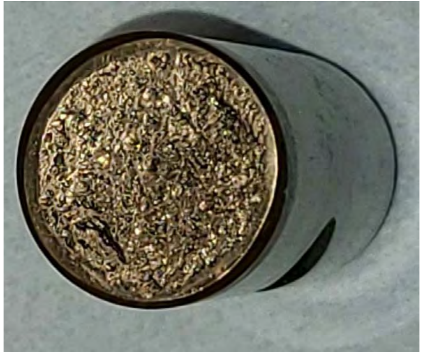
This is the picture of the tappet that matched the warn cam lobe. It is very pitted and was warn in a conical shape that cannot be seen in the photo
