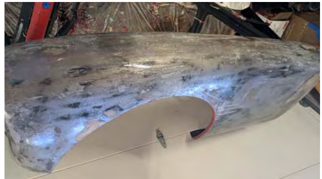
Coopers is expensive for large areas; a Harbor Freight "surface conditioning tool is a cheaper process.
