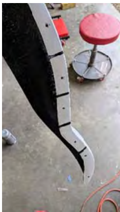
The front valance with sections to allow a flex fit
