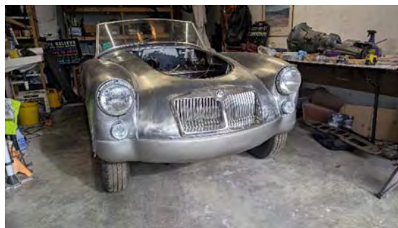
MGA with the front valance installed
