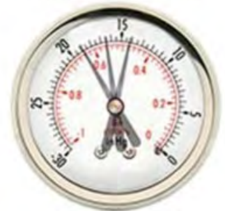
Loose Valve Guide Fast Vibration of needle between 14 and 19
