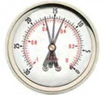
Carb Out of Adjustment Needle floats slowly between 13 and 17
