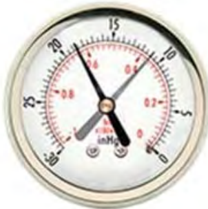
Burnt Valve Needle drops regularly several divisions
