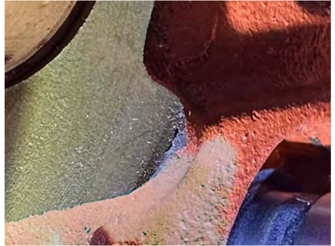
An image of the little excess metal that caused the clicking.
