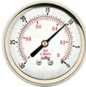
Late Valve Timing Needle reads between 8 to 15 and remains steady
