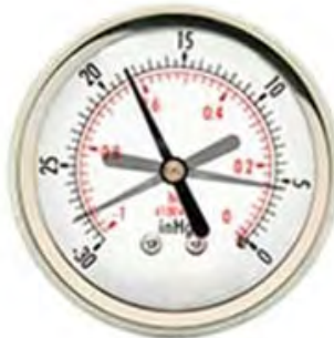
Normal Motor Open and close throttle rapidly rings and valves okay.
