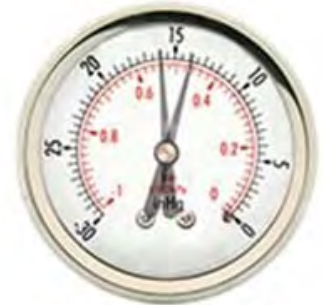
Plug Gap Too Close or Points not Synchronized Needle floats slowly between 14-17
