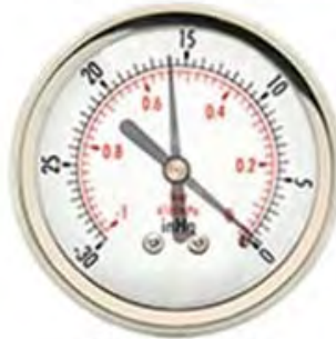
Choked Muffler High reading at first, Breaks to 0 and builds back to 16
