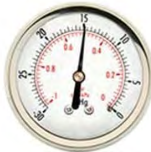
Poor Rings or Oil Needle steady but lower than normal
