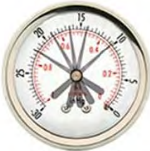
Weak Valve Guides Motor racing, needle registers 10 to 22, variations increase with RPM
