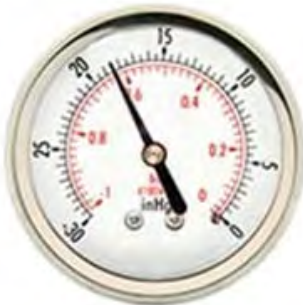
Normal Motor Needle steady between 17 & 21
