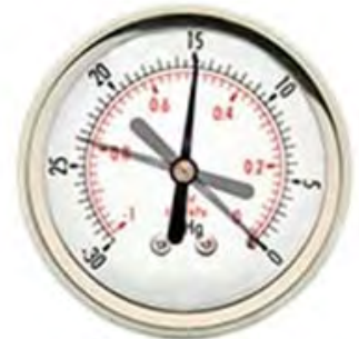
Poor Rings or Oil Open and close throttle rapidly needle pulls down to zero.
