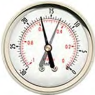
Sticky Valve Needle drops occasionally about 4 divisions
