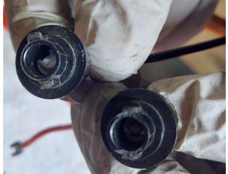
Broken ends of an in-line fuse holder
