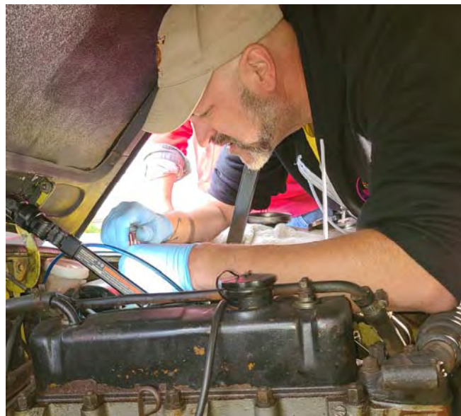
Mathieu cleaning out a stuck float valve.
